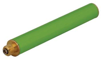
A broadband, rugged, in-building or outdoor antenna designed to service the whole 406-470 MHz UHF band and GSM quad band. With modest dimensions of 25 mm (OD) x 182 mm (height), this antenna radiates with a typical peak omnidirectional gain of +3 dBi. Internally, the radiating element is DC shunted to help protect the transceiver ElectroStatic Discharge (ESD).
